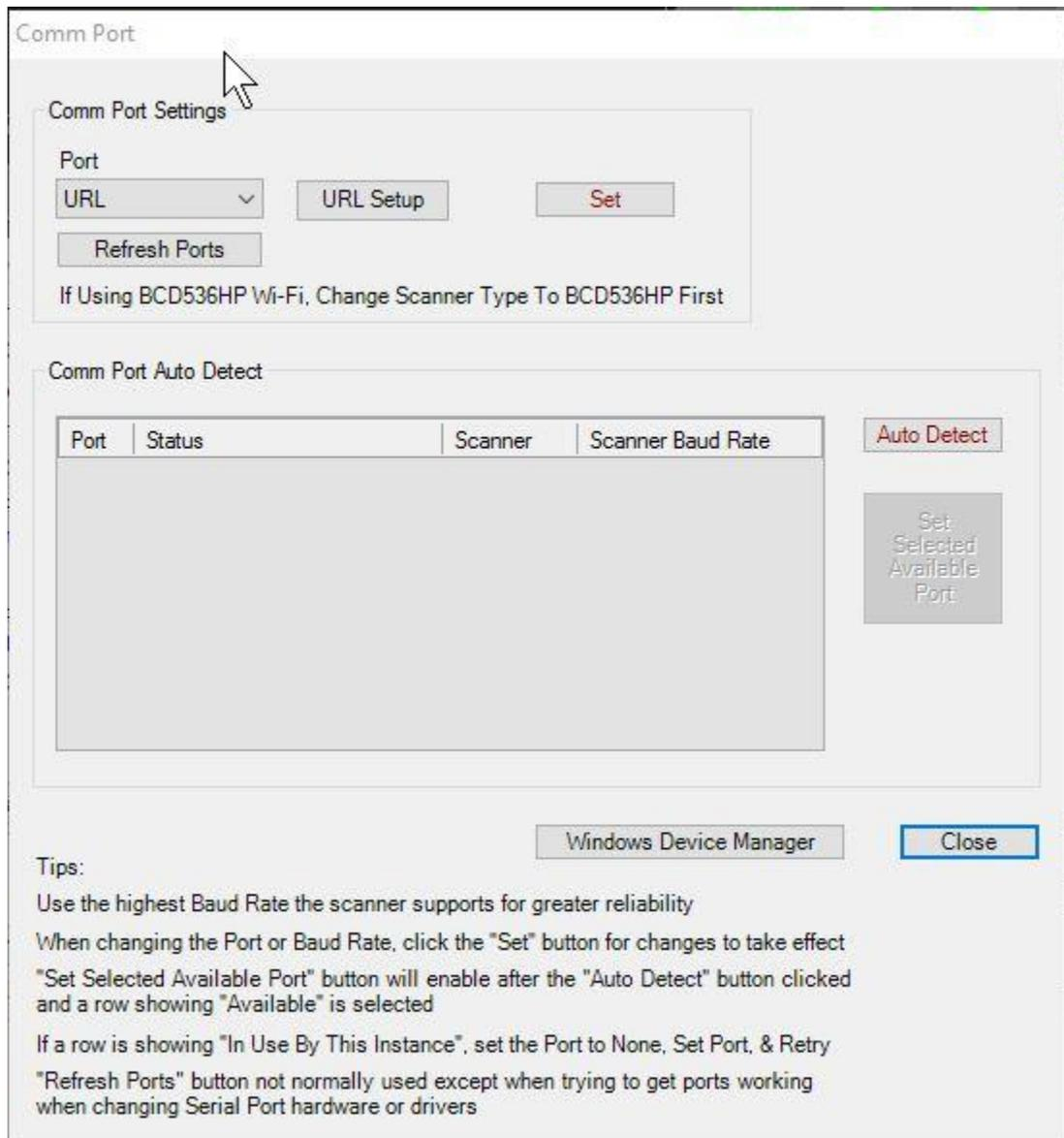
16. Click on the URL Setup button. If you see a RED highlighted UDP Not Connected (see image below), the IP address shown in the URL box is NOT correct. That IP address must match the IP number assigned to the Uniden BCD536HP by your home router. That is the number you wrote down in Section 1, step 7.
