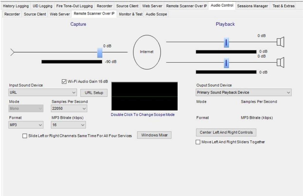
NOTE: This will allow the audio coming from the BCD536HP to be sent with your stream (feed) without having to use any physical audio cable connection between the scanner and your PC. The audio quality using the Wi-Fi method above is superior.
